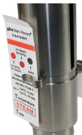
Use of a chemical indicator inside the clip of a combination autoclave, e.g. Sirona DAC UNIVERSAL
