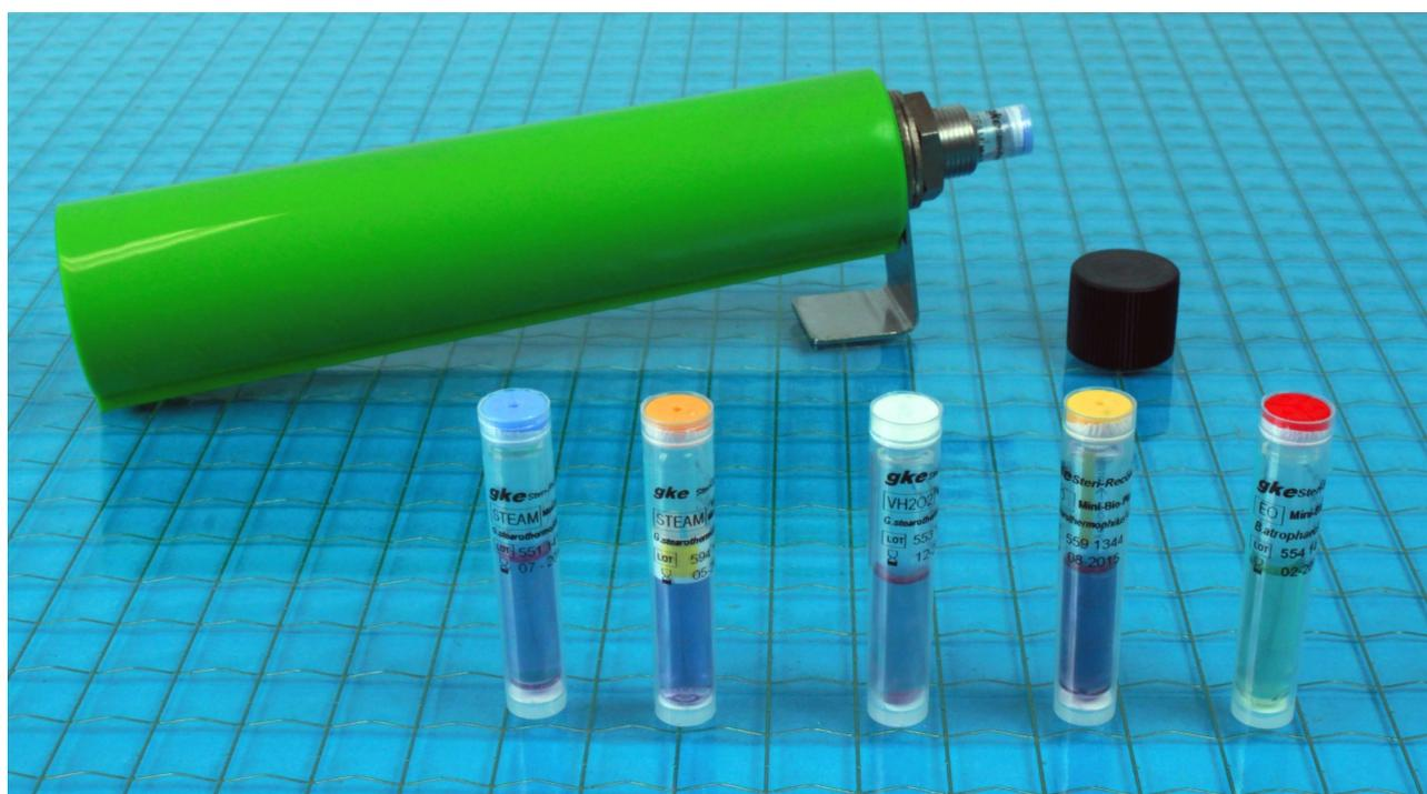
Fig. 1: Mini-Bio-Plus SCBIs and Bio-Compact-PCD®
