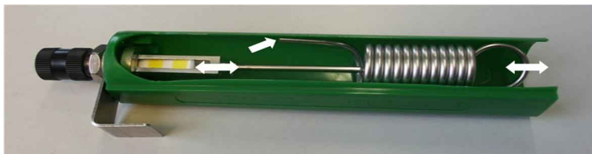
The combination of those 4 connected design elements allows by modifying each of them to produce a variety of different test devices especially tailored to sterilizer type tests or to check special load configurations. This unique design allows to simulate the sterilant penetration characteristic of packed solid instruments, hollow devices and even porous loads, without using porous components using the large volumes as an entrance in the PCD.
