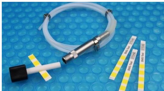
Colour change of the inserted indicator strip with complete and insufficient steam penetration.
