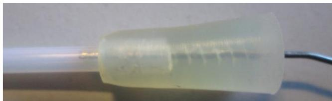
Picture 2 Thermo couple element in a teflon tube
