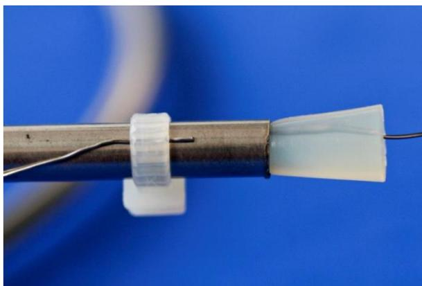
Other thermocouple elements were fixed at the outside wall of the tube and in the free chamber. This way the temperature gradients in the tube, at the outside of the tube and in the sterilizer chamber could be compared.
