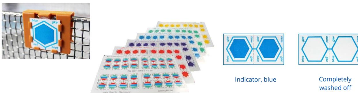
GKE produces cleaning process monitoring indicators, i. e. artificial test soils, which are added to the cleaning process. After the end of the program the indicators can be checked optically for cleaning success.
